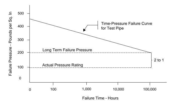
The figure above illustrates the basic method used in assigning Pressure Rating. Note that the assigned Pressure Rating is one half of the long term test failure pressure.
